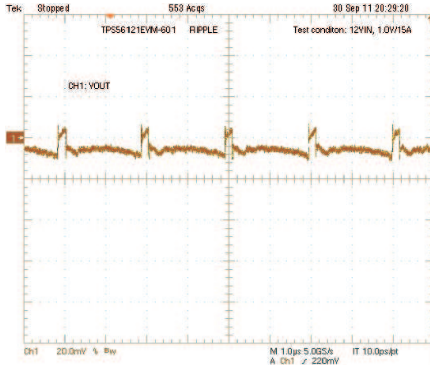
Figure 8. Output Voltage Ripple (V IN = 12 V, V OUT = 1.0 V, I OUT = 15 A)
