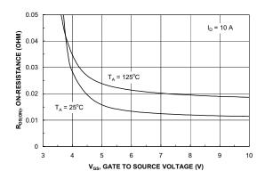
Figure 4. On-Resistance Variation with Gate-to-Source Voltage.
