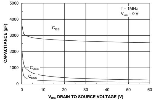
Figure 8. Capacitance Characteristics.
