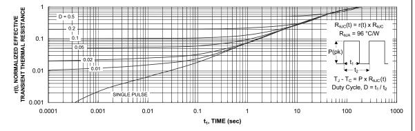
Figure 11. Transient Thermal Response Curve.
