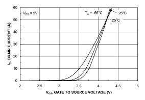
Figure 5. Transfer Characteristics.
