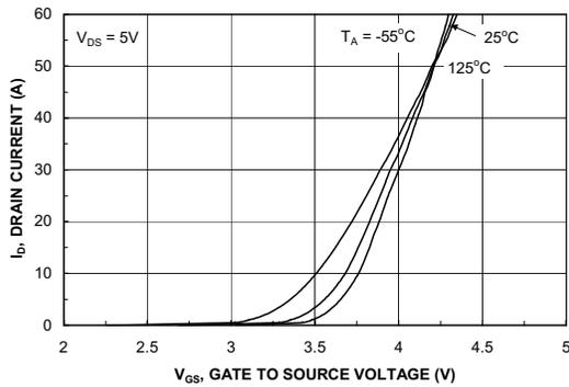
Figure 5. Transfer Characteristics.
