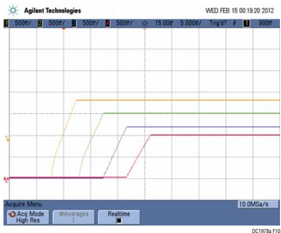
Figure 10. Cascade Sequencing Up with DC1978A
