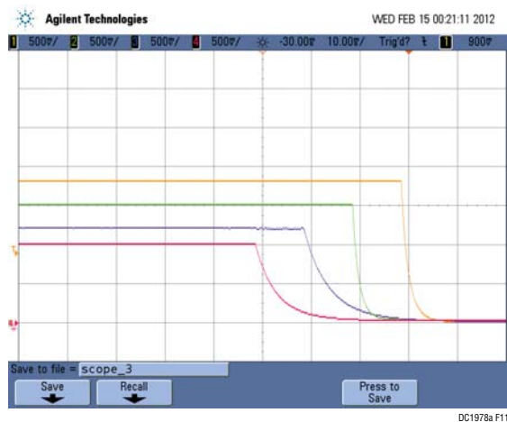
Figure 11. Time Based Sequencing Down with DC1978A
