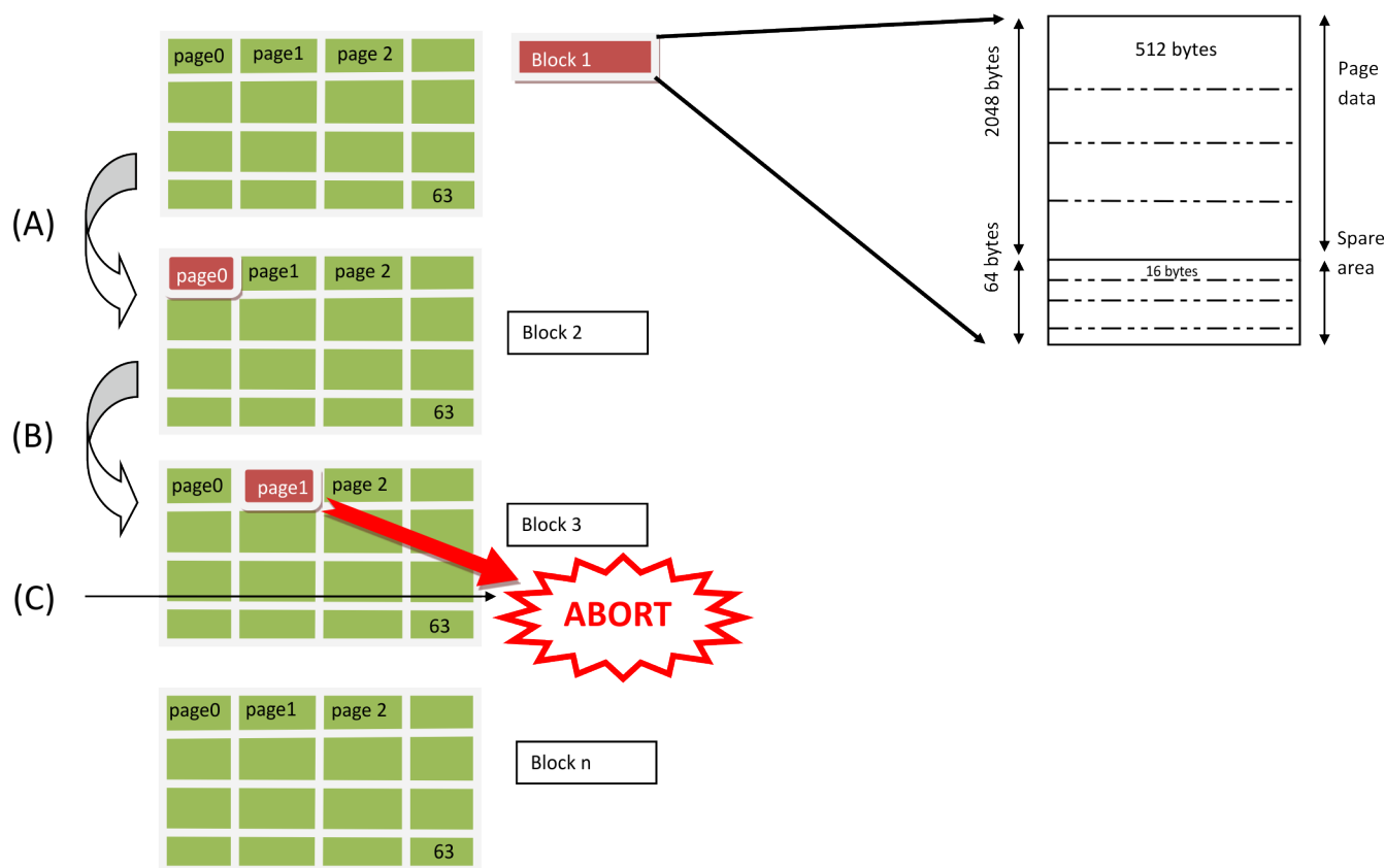
Figure 11. D800K008 ROM Behavior Before Application of Software Patch (1)
