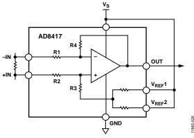
Figure 28. Vs Referenced Output
