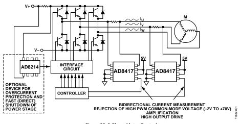
Figure 33. 3-Phase Motor Control
