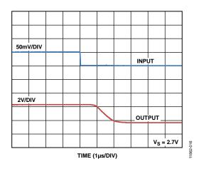
Figure 17. Differential Overload Recovery, Falling ( $V_s = 2.7 V$ )
