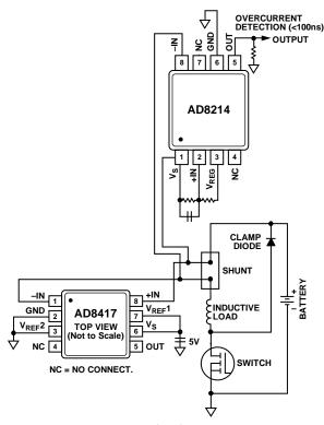
Figure 36. High Rail Current Sensing
