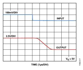
Figure 18. Differential Overload Recovery, Falling ( $V_S = 5 V$ )
