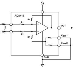
Figure 27. Ground Referenced Output
