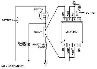
Figure 35. High-Side Switch
