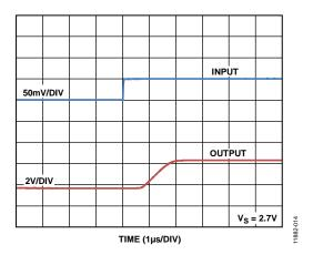
Figure 15. Differential Overload Recovery, Rising ( $V_s = 2.7 V$ )
