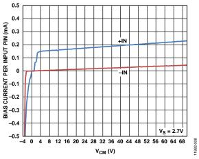
Figure 9. Bias Current per Input Pin vs. V<sub>CM</sub>
