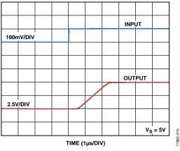
Figure 16. Differential Overload Recovery, Rising ( $V_S = 5 V$ )
