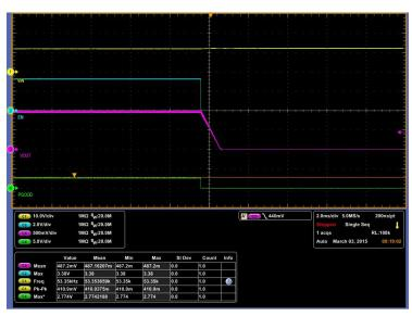
Ch1 =  $V_{IN}$  at 10 V/division, Ch2 = CNTL at 2 V/division, Ch3 =  $V_{OUT}$  at 500 mV/division, Ch4 = PGOOD at 5 V/division Figure 12. Soft Stop from Control, 0.95-V Output at 12  $V_{IN}$ , 20-A Output
