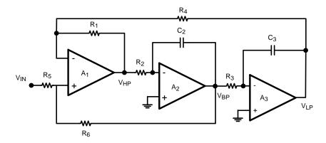
Figure 38. State Variable Active Filter
