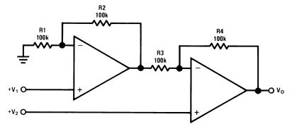
Figure 31. Two-Op-Amp Instrumentation Amplifier
