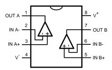
Figure 2. Top View - 8-Pin VSSOP
