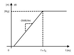
Figure 35. High Pass Filter Transfer Function
