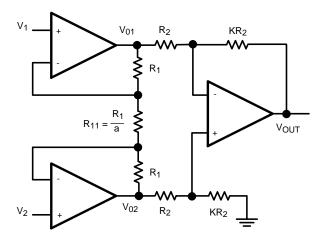
Figure 30. Three-Op-Amp Instrumentation Amplifier
