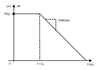
Figure 33. Low Pass Filter Transfer Function
