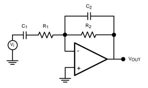
Figure 36. Band Pass Filter
