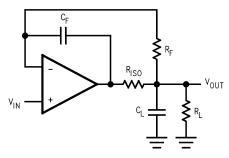
Figure 27. Indirectly Driving a Capacitive Load with DC Accuracy
