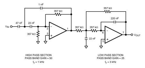
Figure 1. High Gain Band Pass Filter
