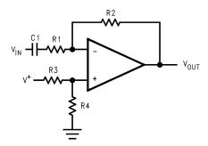
Figure 29. Single-supply Inverting Amplifier
