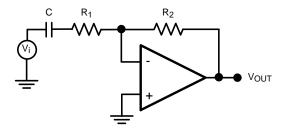
Figure 34. High Pass Filter
