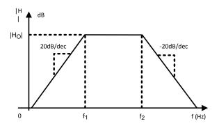
Figure 37. Band Pass Filter Transfer Function
