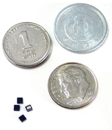
INA300 is in a tiny 2mm x 2mm QFN package minimizing footprint requirements.
