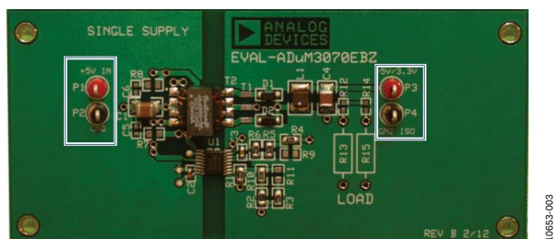
Figure 3. Single Supply Terminals
