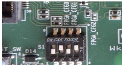
Figure 20. FPGA Config Switch
