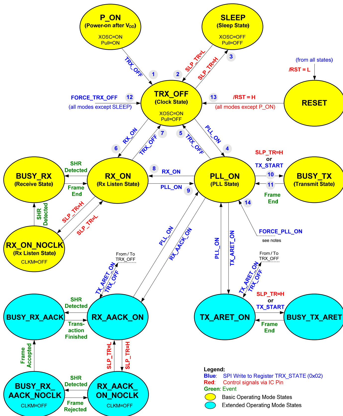
Figure 5-8. Extended Operating Mode State Diagram
