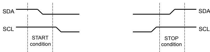
Figure 14-3. START and STOP Conditions
