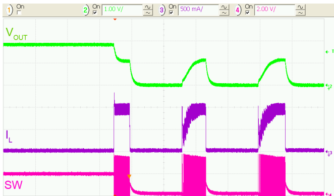
Figure 35. Over-Current Fault Response, R_{LOAD} = 1\text{ }\Omega , 50\text{ }\mu\text{s/div.}
