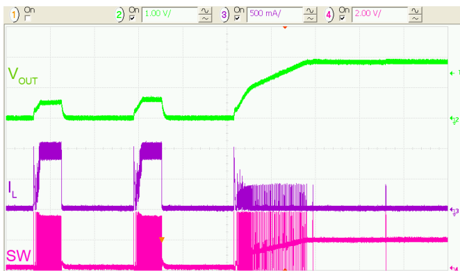
Figure 37. Overload Recovery to Light Load, 50\text{ }\mu\text{s/div.}
