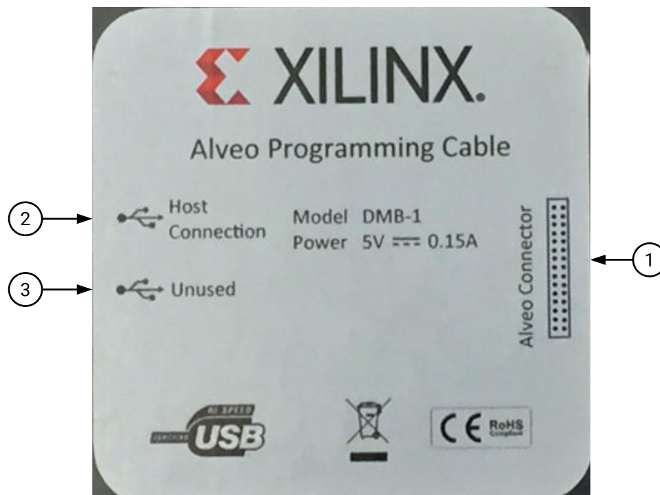
Figure 1: Alveo Programming Module Interface Locations
