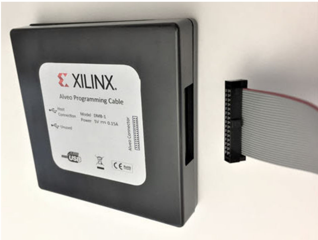
Figure 3: Connecting Ribbon Cable to Debug Connector
