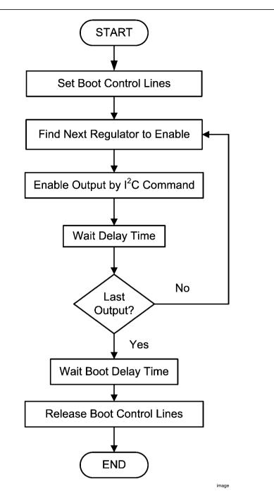
FIGURE 7. MCU Output Enable Routine Flow Chart
