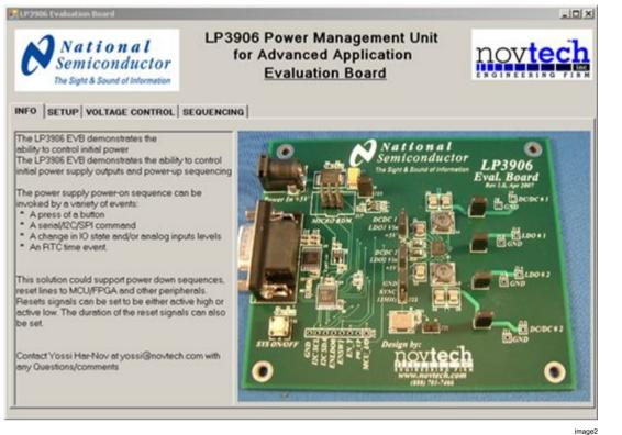
FIGURE 8. LP3906EBV Advanced Application Board PC Control Software - INFO Panel
