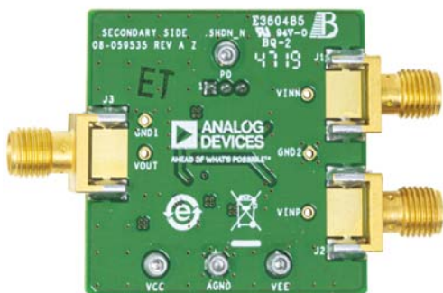
Figure 2. EVAL-LTC6226S8/EVAL-LTC6228IS8, Secondary Side
