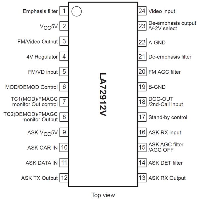
Figure 1. Pin Assignment
