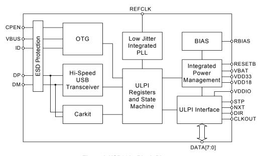
Figure 1 USB3317 Block Diagram
