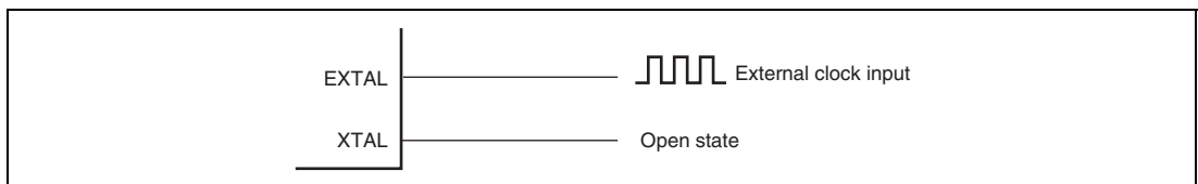
Figure 4.4 Example of External Clock Connection
