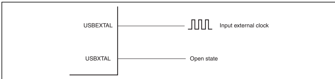
Figure 4.6 Example of Connecting an External 48-MHz Clock
