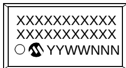
14-Lead SOIC (3.90 mm)
