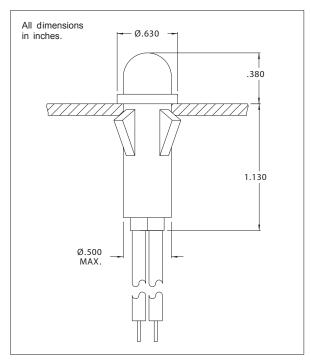
Solid-state indicator lights complete with built-in current-limiting resistor and rectifier diode.
