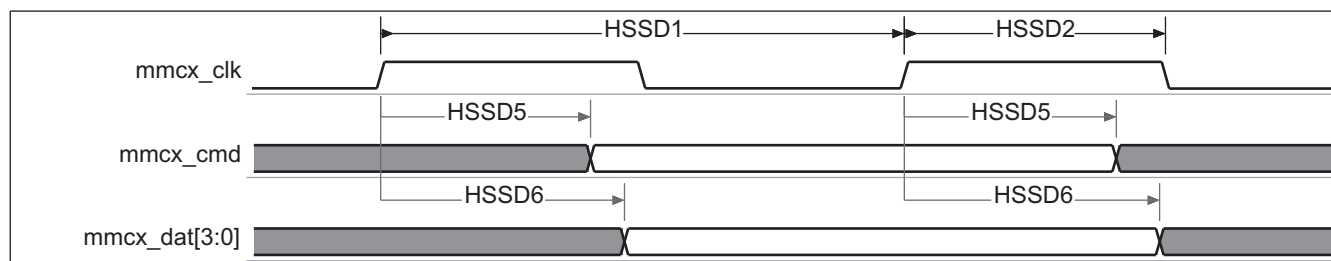
Figure 6-66. MMC/SD/SDIO – High-Speed SD Mode – Data/Command Transmit
