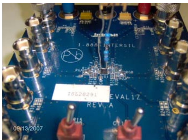
FIGURE 8. IMPROVED ANTENNA DESIGN TO EVALUATE RADIATED INTERFERENCE
