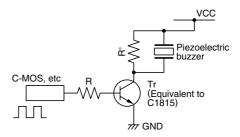
\* Resistor to do charging and discharging to a piezoelectric element (Value of about  $1k\Omega$  is good efficiency).
