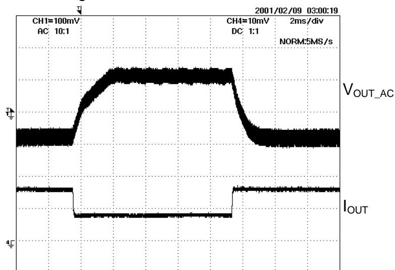
Figure 17. Transient Response 265 V AC 50 Hz, I OUT : 0.03 A to 0.33 A V OUT & I OUT (100 mV & 200 mA/div, 2 ms/div)
