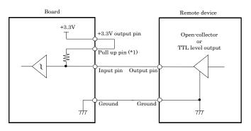
$^*$ 1 : The pull-up pins are PUP1 for the counter input signal and PUP2 for the control input signal.  $\bigwedge$  CAUTION
