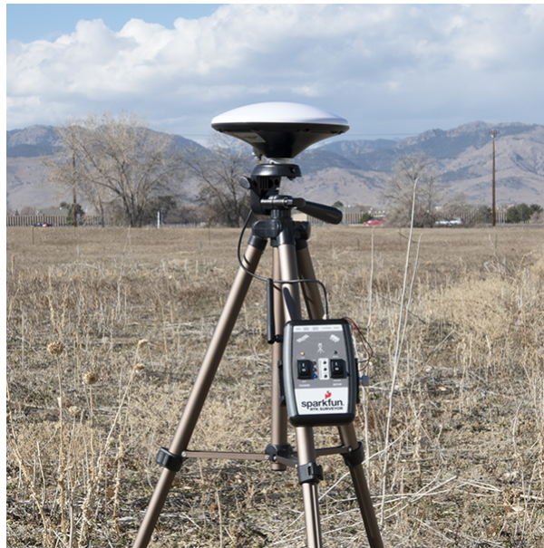
Temporary RTK Surveyor Base setup
