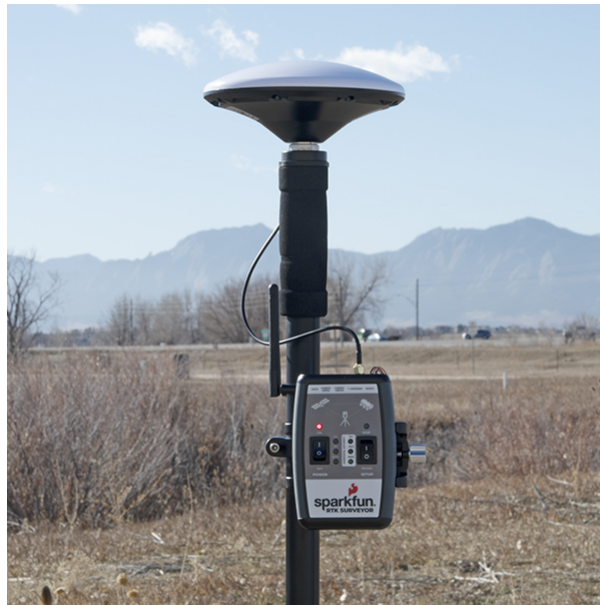
2nd most common setup with a 915MHz Radio providing RTCM
