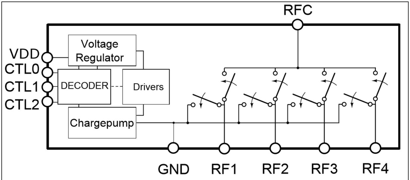
**Figure 1** BGSA143GL10 Block diagram
