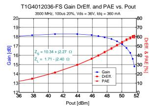
120W Peak Power, 24W Average Power, 36V DC – 3.5 GHz, GaN RF Power Transistor
