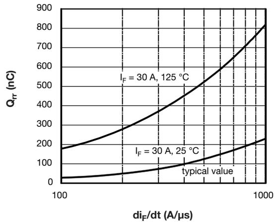
Fig. 8 - Typical Stored Charge vs.  $di_F/dt$
