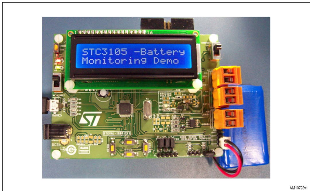
Figure 1. STEVAL-ISB012V1 single cell Li-Ion battery monitor and gas-gauge based on the STC3105
