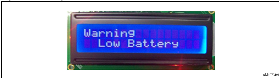
Figure 9. Battery low indication
