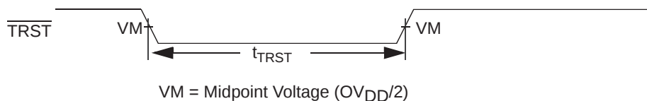
Figure 20. \overline{TRST} Timing Diagram
