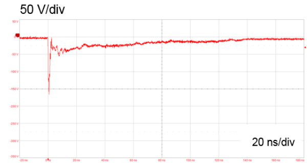
Figure 5. ESD response to ISO10605-C = 150 pF, R = 330 \Omega (-8 kV contact discharge)
