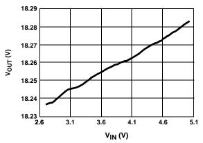
FIGURE 10. LINE REGULATION (I<sub>OUT</sub> = 30mA)
