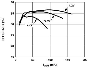
FIGURE 4. EFFICIENCY vs  $I_{OUT}$  ( $V_{OUT}$  = 12.6V) L = 6.8µH (TDK RLF7030) C = 6.6µF
