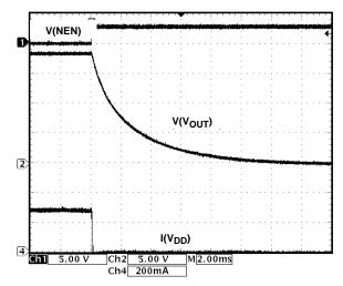
FIGURE 8. SHUTDOWN (V<sub>DD</sub> = 3.6V, R<sub>L</sub> = 360 $\Omega$ )
