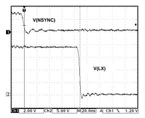
FIGURE 15. NSYNC TO LX SYNCHRONIZATION DELAY
