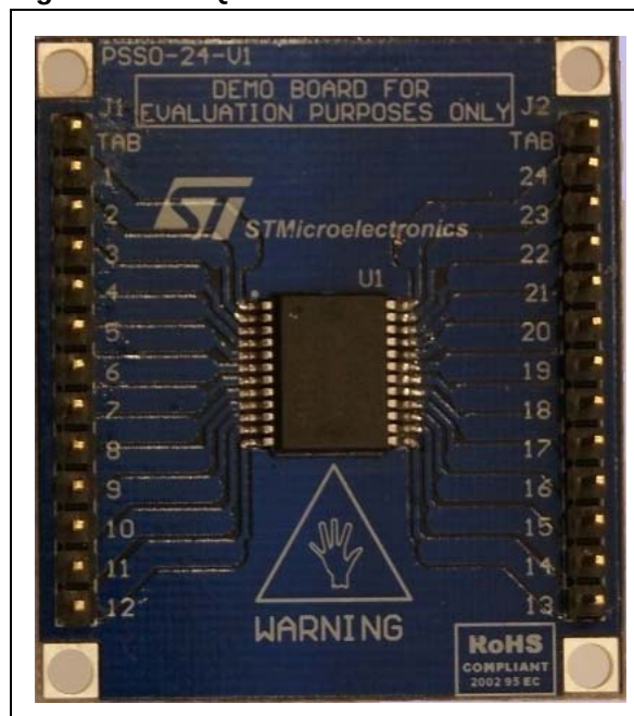
Figure 1. VNQ5E050K evaluation board
