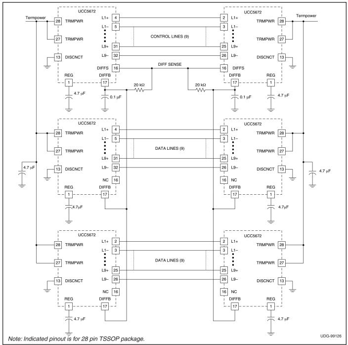
Figure 1. Application diagram.
