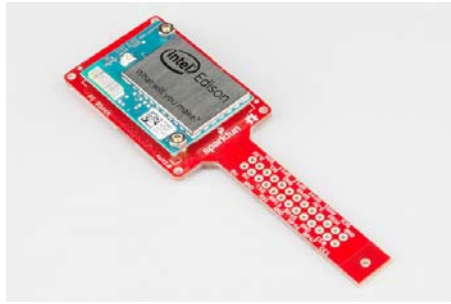
Edison installed on Pi Block
