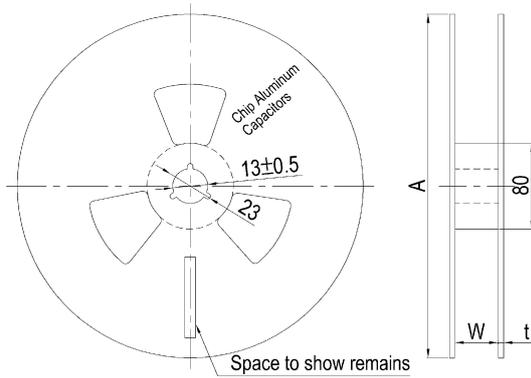
Fig. 2-2 Reel Polarity
