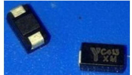
Molded plastic glass passivated junction.
