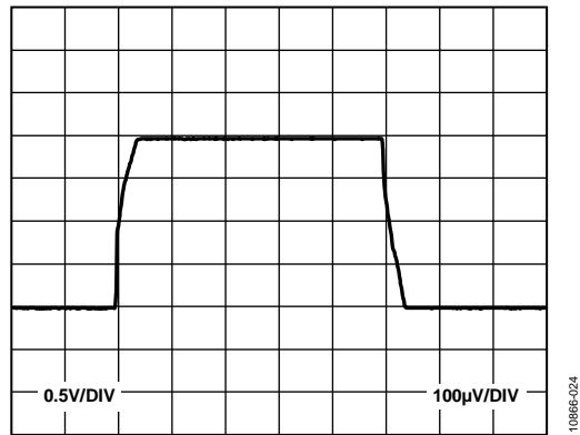
Figure 24. Operational Amplifier Large Signal Transient Response
