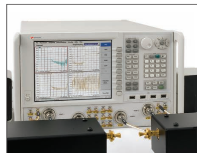
Direct connection of VDI modules to a 50 GHz PNA-X enables S-parameter measurements to 1.05 THz.
