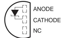
LP (TO-92/TO-226) PACKAGE (TOP VIEW)
