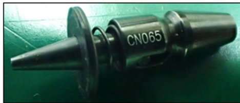
Samsung off-the-shelf nozzle model: CN065 Nozzle tip material: ceramic (zirconia) Nozzle inner diameter: 0.65 mm Nozzle outer diameter: 1.20 mm
