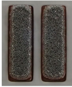
Figure 7. An example of a good stencil printing on PCB.
