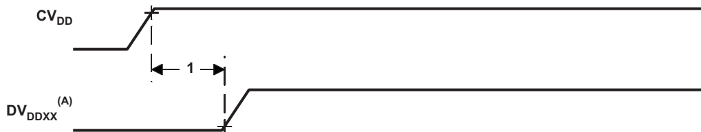
Figure 6-5. I/O Supply Timings
