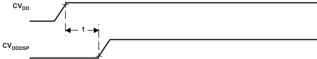
Figure 6-4. DSP Host-Boot Mode Core Supply Timings
