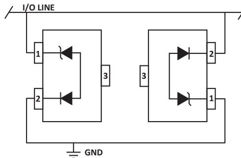
**FIGURE 1 - COMMON MODE I/O PORT PROTECTION**
