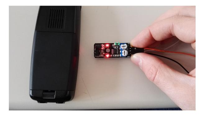
This sensor allows you to activate and deactivate the obstacle detection by manipulating the enable-pin. It is activated by default which means that the sensor is in detection mode by default.
