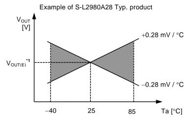
\*1. V<sub>OUT(E)</sub> is a mesured value of output voltage at 25 °C.
