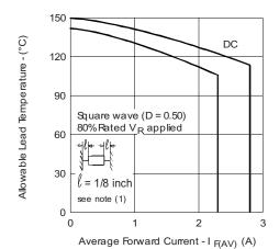
Fig. 4 - Maximum Allowable Lead Temperature vs.
