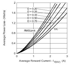
Fig. 5 - Forward Power Loss Characteristics
