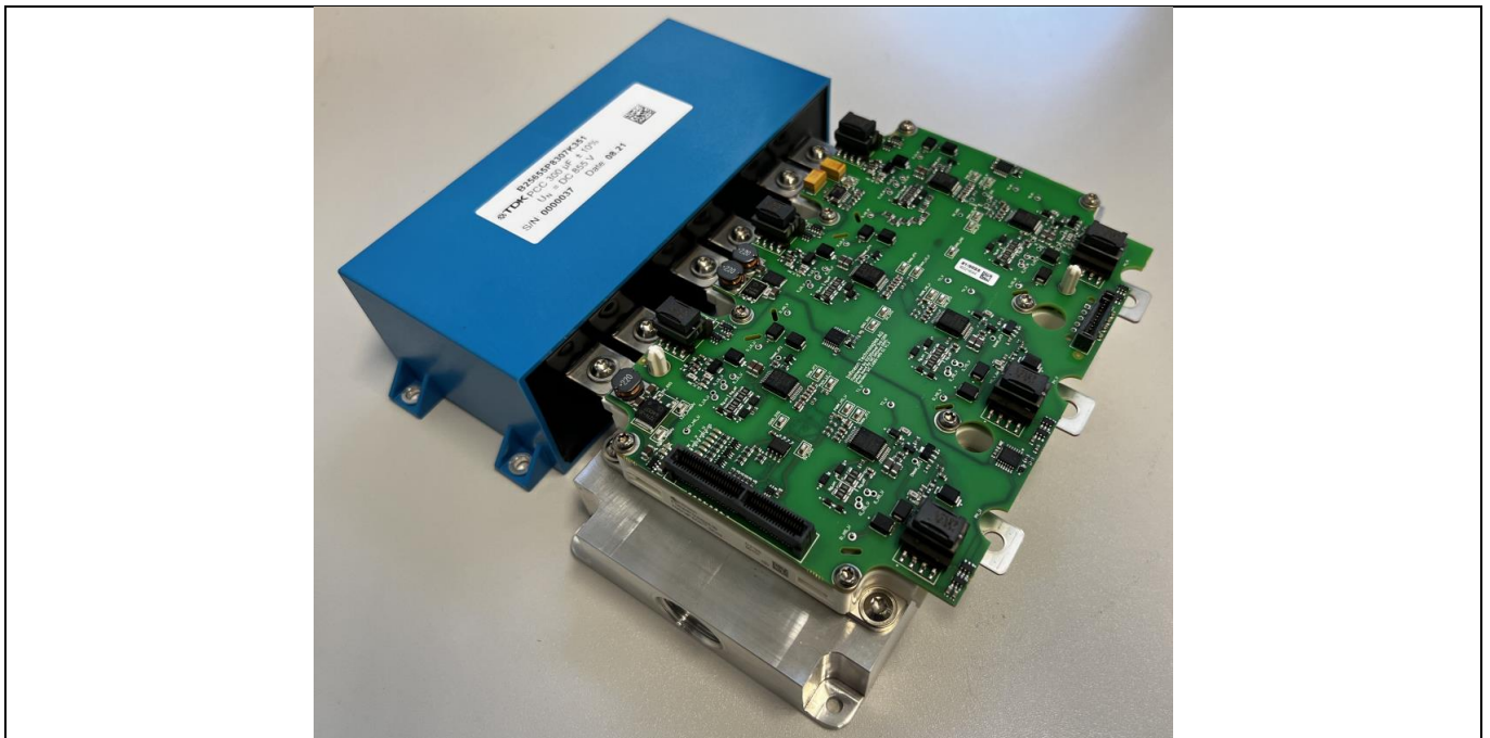
Figure 1 Typical appearance of the evaluation kit EVAL KIT HPD G1 SiC SP005594933.
