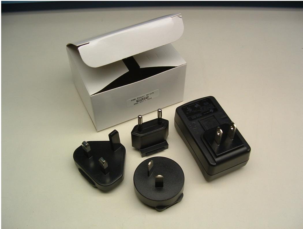
Figure 3-5. USB power supply with interchangeable AC adapters
